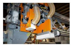
Saw with dust removal system for shaping the frame covers
