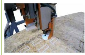
Milling or drilling heads to make holes for cables, openings for windows, doors or create other recesses
